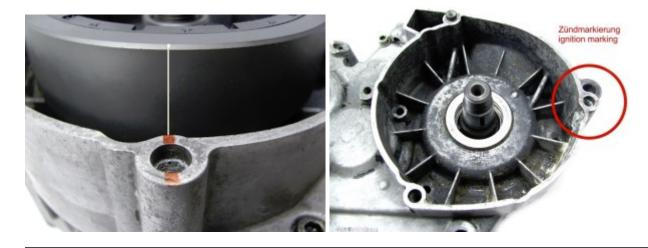
Unscrew the new statorcoil from its base (3 screws M4) to get access to the screw holes on the base. Take care not to demage the paint insulation.
