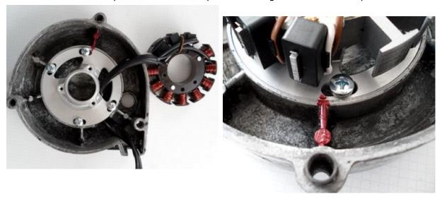
Now everyting is geared up. You may place the cover back on. Put the spark plug back. Double checking that the flywheels magnets have not caught any foreign objects (washers, screws etc).
