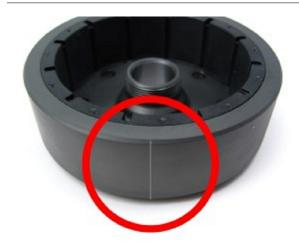
Have a look at the new rotor. You will find on its circumference equally some marking (a pressed or lasered in line).
