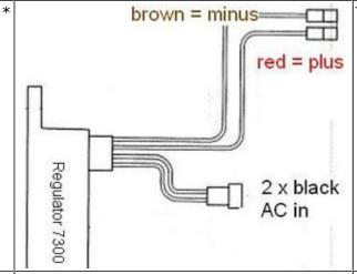
The new regulator/rectifier has 4 wires
