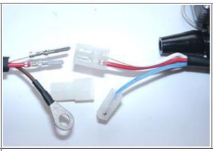
Look for the ignition coil with its female plug and the two wires (red and white).
