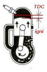
Set the crankshaft (if needed by help of the provisionally fitted new flywheel) into ignition position. This should be for Type 366 (370cc) and Type 406 (399cc) 2.5mm BTDC (20-degrees +/- .2-degrees), for Type 244 and 280 (248cc and 277cc) as well as Type 124 (124cc) and Type 174 (173cc) 1.3mm (15-degrees+/- .1-degrees).
