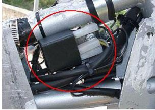
Wiring for racing system is simpler, but basically same as for lighting system, only that regulator does not exist. Nor exist the 2 black wires running from the stator (to the regulator).
